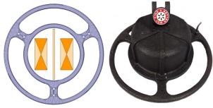
Fig. 1. Photograph of a typical dual-modality detector and an image of the placement of the GPR antennas.
