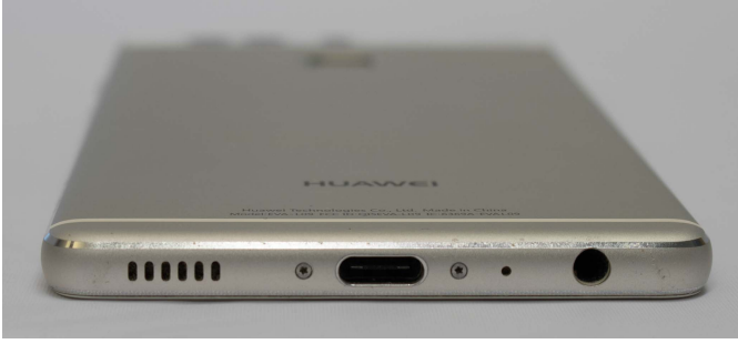
Fig. 1. mm-wave module may be disguised as speaker slots that are already present in smartphones, such as the Huawei P9.
