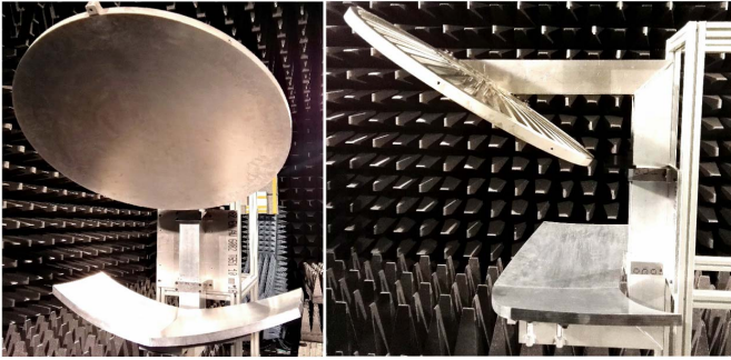
Fig. 22. Photograph of the prototype using a complex offset double reflector setup.
