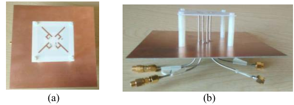
Fig. 12. Photographs of the fabricated four-port DPSD antenna without feed network. (a) Top view. (b) Side view.
