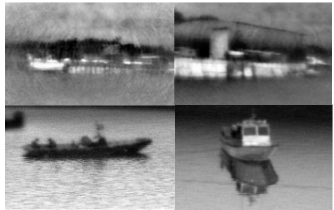
Fig. 4. Measured imagery in the horizontal polarization showing a metal boat with brick buildings in the background (top left) [54], metal pilings (top right) [54], a rubber boat (lower left) [53], and a fiber glass boat (lower right) [52]. Black denotes radiometrically ‘hot.’
