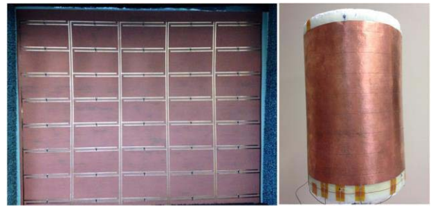
Fig. 15. Fabricated bias circuit on the substrate and the final antenna.
