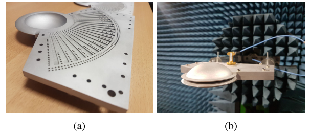
Fig. 8. (a) Photograph of the prototype. (b) Measurement setup in the anechoic chamber.
