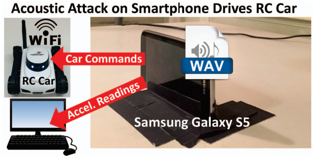
Figure 13. Smartphone Attacking its own Accelerometer to Control an RC Car. An Android phone runs an application that controls an RC car based on the phone’s orientation, measured by its internal MEMS accelerometer. Simultaneously, a malicious audio file is playing over the phone’s speaker, mounting an output control attack on the phone’s accelerometer. The RC car is essentially piloted by the audio file.
