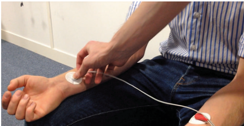
FIGURE 3. A convenient placement of electrodes on the forearms, for the recording of the ECG.
