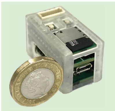
FIGURE 4. Our iAmp recording device against one U.K. pound coin (22.5 mm in diameter).
