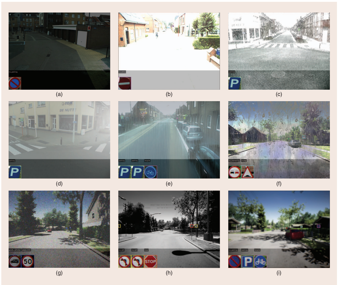
FIGURE 1. Examples of challenging conditions in a scene from the 2017 VIP Cup: (a) darkness, (b) brightness, (c) snow, (d) haze, (e) rain, (f) dirty lens, (g) noise, (h) decolorization, and (i) blur.
