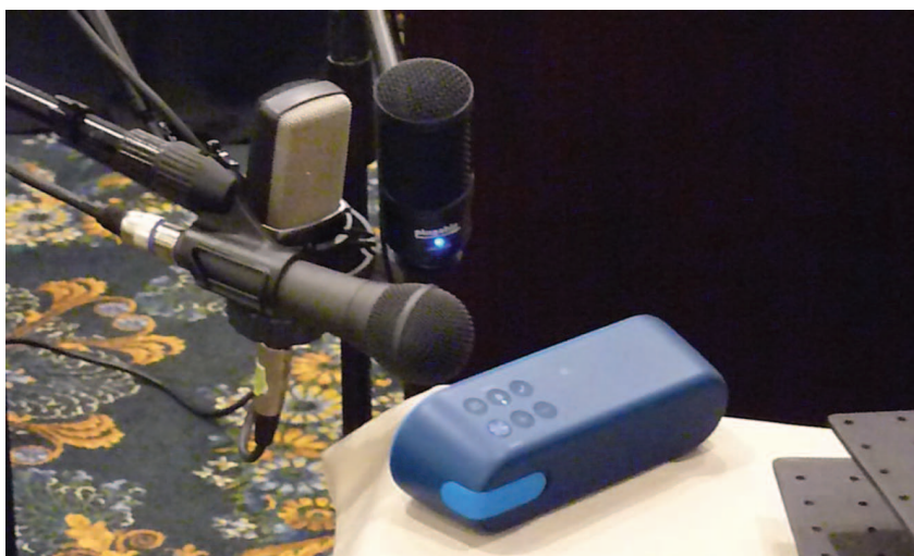
FIGURE 2. A Real-time beat-tracking assessment for the final competition: music was played from the Bluetooth loudspeaker and recorded by three microphones, one for each team.
