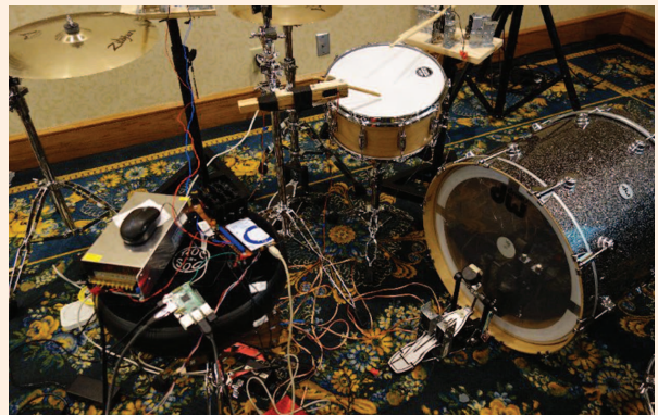
FIGURE S3. The automated drums for Team Madmom and Team Beats on the Barbie. Both teams implement drum signals for the bass drum, the snare drum, and the hi-hat.
