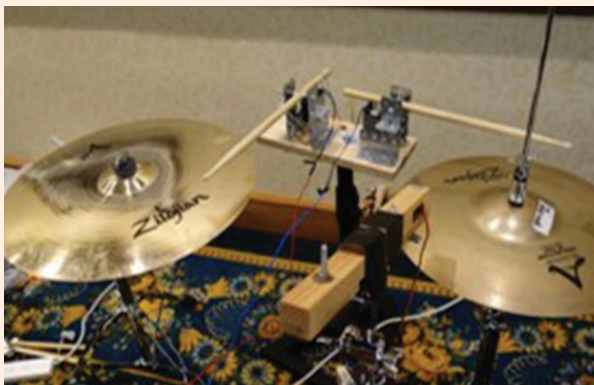
FIGURE S2. Solenoid-based actuators for Team Beats on the Barbie.
