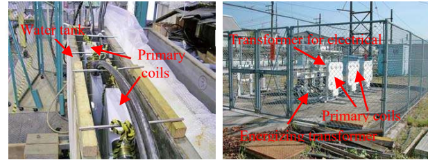
(b) Test device for long term outdoor test
