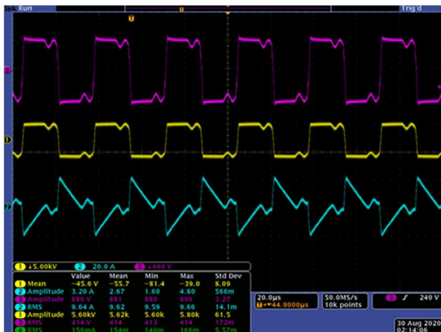
Fig. 14. Primary Voltage (Probe 3) and Current (Probe 2), and Medium Voltage 5.6kV (Port 1)
