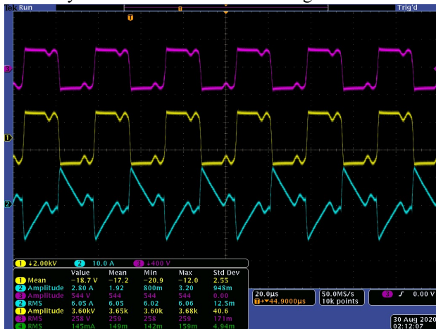
Fig. 13. Primary Voltage (Probe 3) and Current (Probe 2), and Medium Voltage 3.6kV (Port 1)
