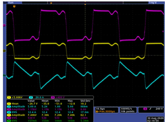
Fig. 15. Primary Voltage (Probe 3) and Current (Probe 2), and Medium Voltage 7.4kV (Port 1)
