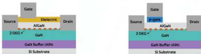
Fig. 4. The cascode depletion-mode (left) and enhancement-mode (right) of GaN power devices [54].
