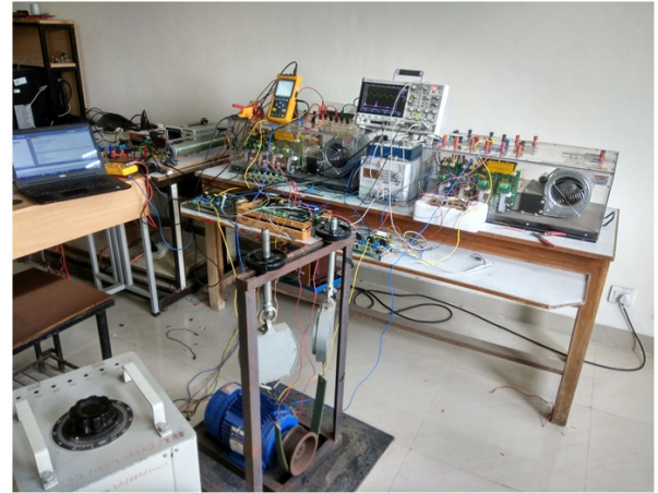
Fig. 9. Test setup of SPAIM fed by D3VSIs.
