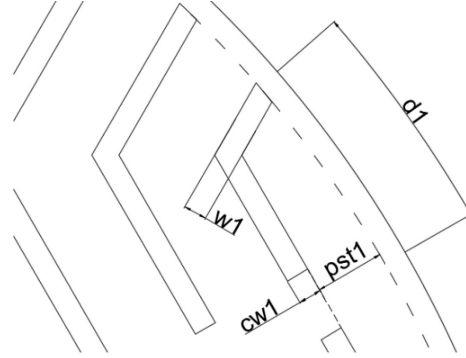
Fig 5. New rotor geometry of 1st flux barrier.
