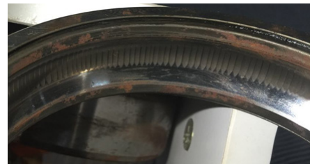
Fig. 5. Bearing ring damage caused by CM current.
