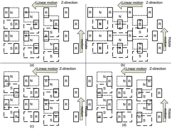
Fig. 5. Operation model of the new FSTFMaLM in the rotate model and the linear model.
