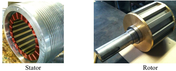
Fig. 18 Prototype SRM for traction [45]
