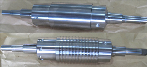
Fig. 12. Smooth and circumferentially grooved rotors of a 10kW, 70krpm PM BLDC machine developed by ZJU.
