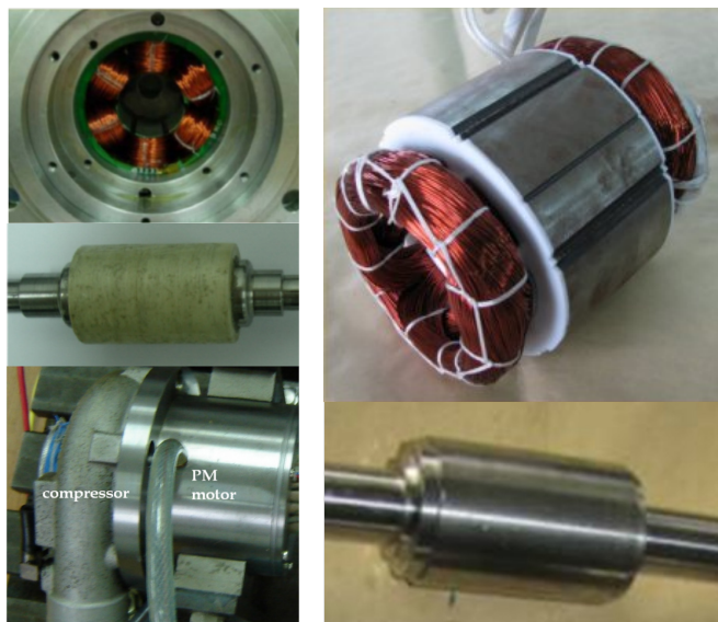
(a) A 3kW 120krpm PM motor for air compressor developed by ZJU (b) A 20kW 70krpm PM motor for conditioning compressor developed by ZJU
