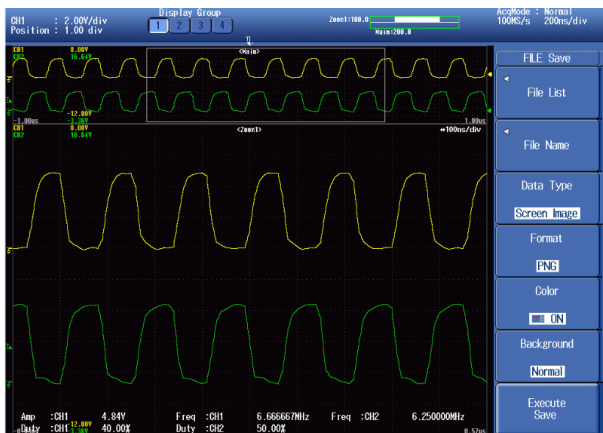
Fig. 14. The gate signals of two complimentary GaN HEMTs in the same leg.
