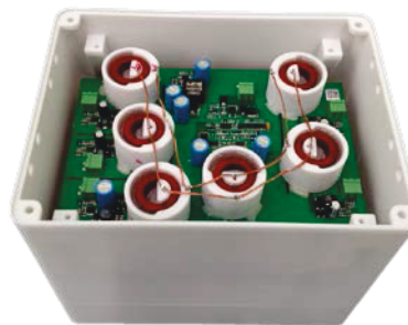
Fig. 10. Solar inverter cell using 10 kV SiC MOSFET.
