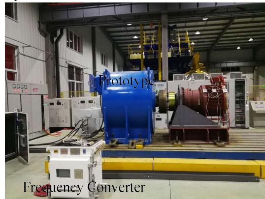
Fig. 7. Prototype temperature rise experimental platform.
