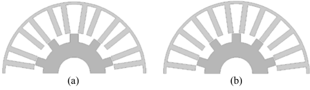
Fig. 7. WFSF machines with different DC to armature slot area ratios. (a) S_f/S_a=1.5 . (b) S_f/S_a=1 .
