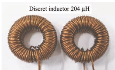
Fig. 8 Two discrete symmetrical inductors
