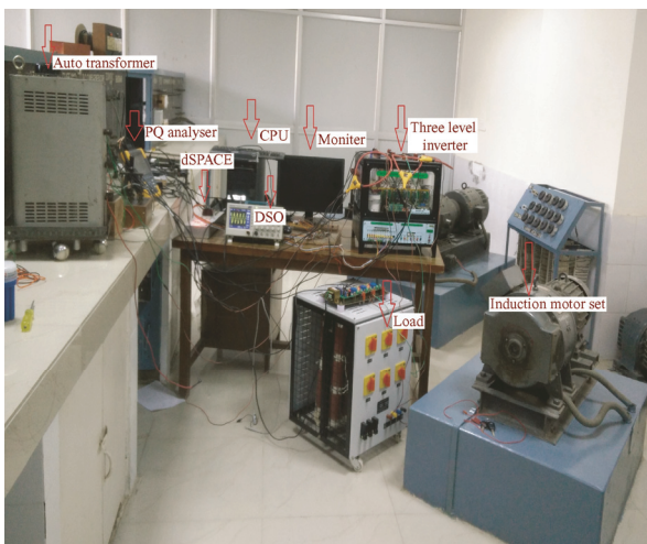
Fig. 6 Pictorial view of the experimental setup for sensorless speed controller
