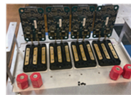
Fig. 10 Two CHB cells
