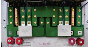
Fig. 11 Hardware design for 2 H-bridges
