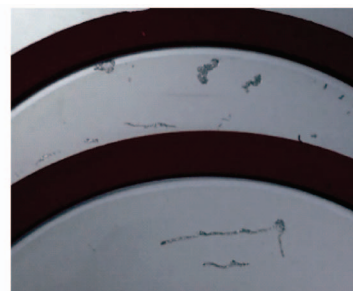
(c) Local burnout under unequal mounting force
