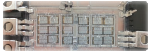
Fig. 18 Power module with nine dies paralleled and a neat waveform [38]
