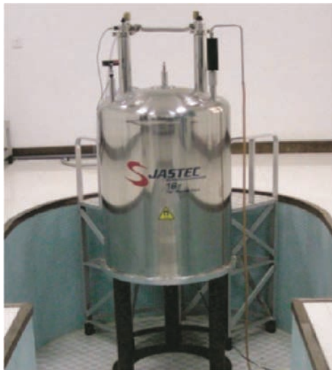
(a) Image of a superconducting magnet providing large gradient static magnetic field
