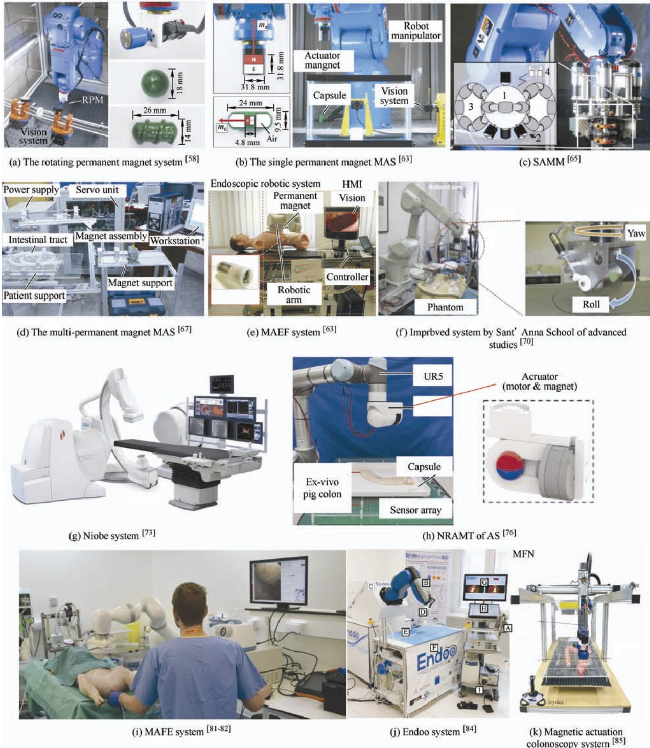
Fig. 4 Permanent magnet MASs using robotic arms
