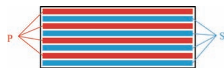
Fig. 14 Staggered winding structure
