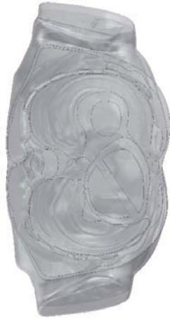
Figure 3. A cross-sectional cut of the torso CAD model passing through the ventricles. It is possible to distinguish the tissues considered for the simulation. From the outer to the inner: The connective tissue, the muscles, the sternum, the costal cartilage, the inflated lungs, the liver, and finally, the heart with its ventricles.
