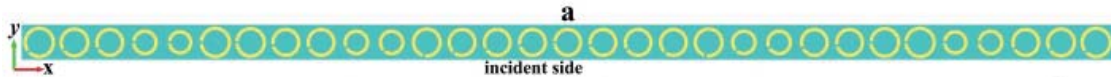
Figure 2a. The design, theoretical, and numerical characterization of the first bifocal metalens with lateral alignment of two foci: a top view of half the metalens layout with a total of M \times N = 16 \times 1 pixels distributed along the x and y axes.
