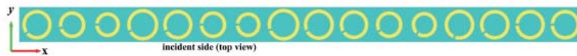
Figure 3a. The design, theoretical, and numerical characterization of the second bifocal metalens with axial alignment of two foci: the top view of the metalens layout with a total of M \times N = 31 \times 1 pixels distributed along the x and y axes.
