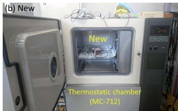
Figure 10b. The temperature test setup for the new ASIC receiver.
