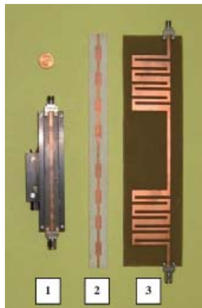
Figure 2 b. Various experimental modules based on planar photonic crystals used at the operating frequencies: f_1 = 9.5 GHz (1), f_2 = 3.2 GHz (2), and f_3 = 1.0 GHz (3).
