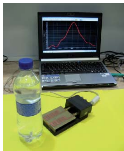
Figure 11. A photo of the (a) finger-shaped module based on planar photonic crystals; (b) portable laboratory prototype for identification and recognition of liquids in closed containers.
