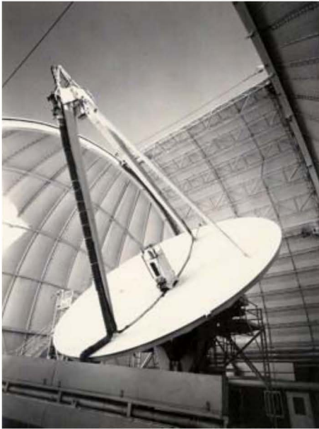
Figure 11. The 36-ft (11 m) millimeter radio telescope of NRAO in its astrodome at an altitude of 2000 m at Kitt Peak Observatory near Tucson, Arizona. Operation started in 1968 (NSF/AUI/NRAO).
