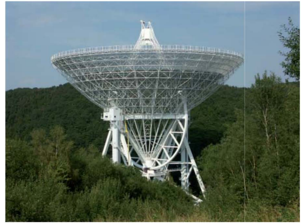
Figure 5b. A photograph of the 100-m telescope of the Max-Planck-Institut für Radioastronomie in Effelsberg, Germany. The telescope performs well at 7 mm wavelength, and acceptably at 3.5 mm (MPIfR).
