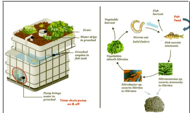
Fig. 2. Aquaponics technique overview (Taken from: abundance.org)
