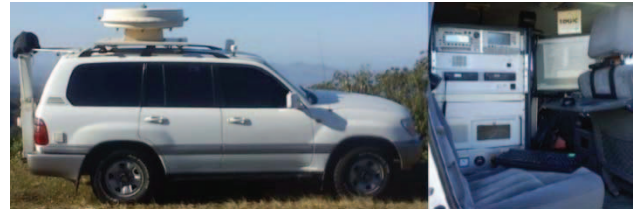
Fig. 4. TELCOR's mobile monitoring unit, outside view (left) and inside view (right).
