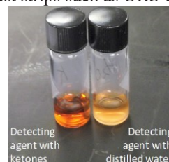
Fig. 5: Test tubes containing 100 \mu L of ketone detection assay each. Left: 100 \mu L of acetoacetic acid at a concentration of 50 mg/mL was added to the ketone detecting solution. Right: distilled water was added at a 1:1 ratio to the ketone detection reagents.
