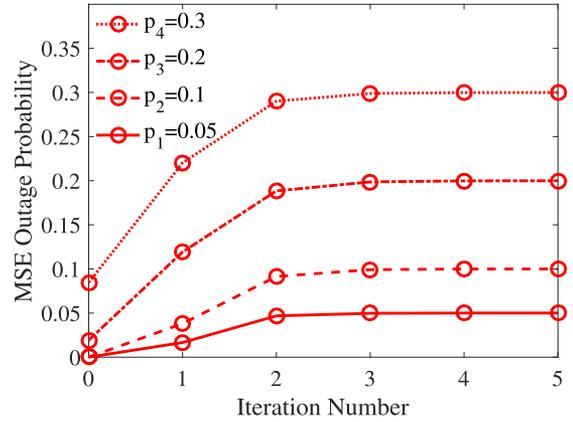
Fig. 5. The convergence performance of the set squeezing procedure for four users.
