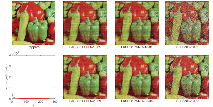
Fig. 5. Row 1: n = 300 ; row 2: n = 400 . Column 1: The true image (peppers) and the singular values of its red channel (which indicates approximate low-rankness); column 2: Lasso with noisy unquantized data; column 3: Lasso with noisy quantized data; column 4: Least squares estimation with noisy quantized data.
