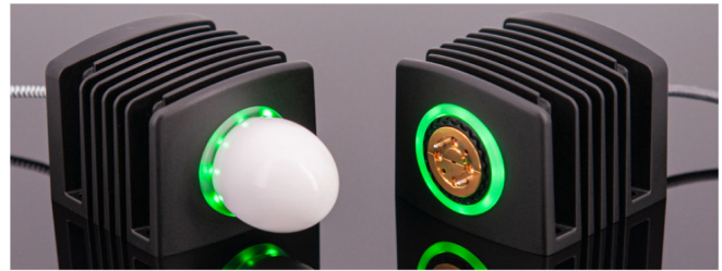
Fig. 1. Photographs of the FMCW radar sensor with dielectric lens antenna (left) and WM-1651 (WR6) waveguide flange (right).
