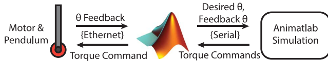
Fig. 5. Schematic representation of information flow between software and hardware platforms. MATLAB manages the communication between the motor/pendulum system and the neural controller in Animatlab.
