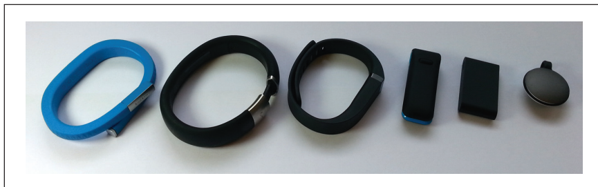
Figure 2. Activity trackers (from left to right): Jawbone's UP, Nike's Fuelband, Fitbit's Flex, Fitbit's Ultra, Withings' Pulse, and Misfit's Shine.
