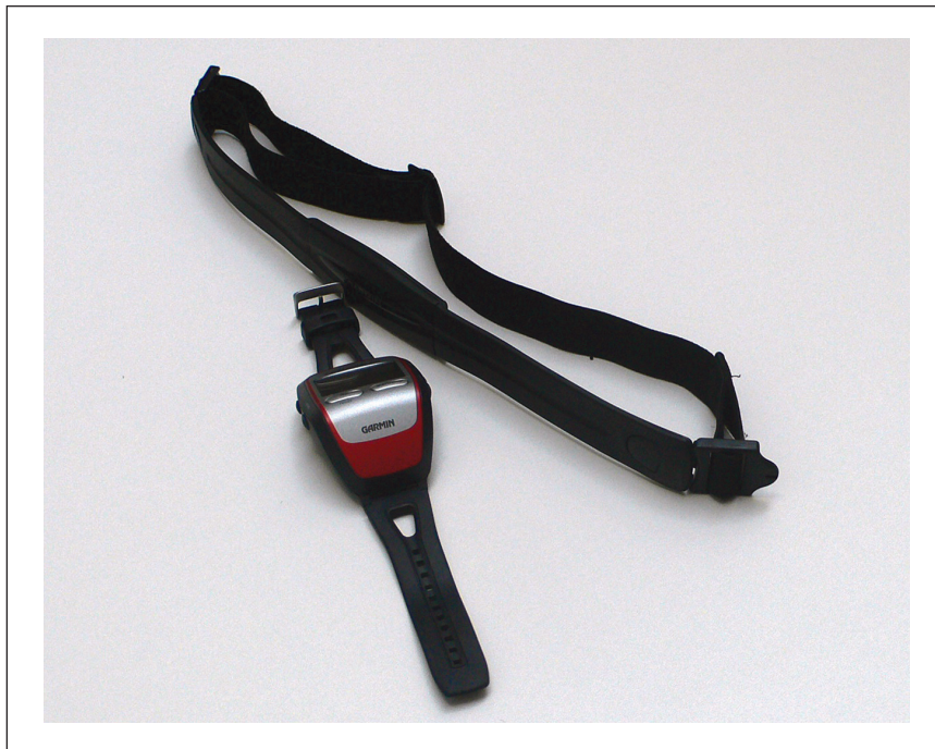
Figure 1. The Garmin Forerunner 305 sports watch. Training watches combine heart-rate monitoring and GPS tracking.
