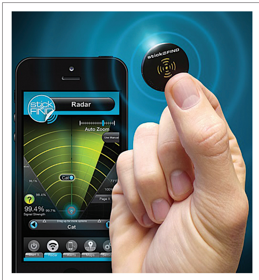
Figure 1. StickNFinds are small Bluetooth devices that you can attach to anything and then find using your smartphone. (Source: StickNFind; used with permission.)
