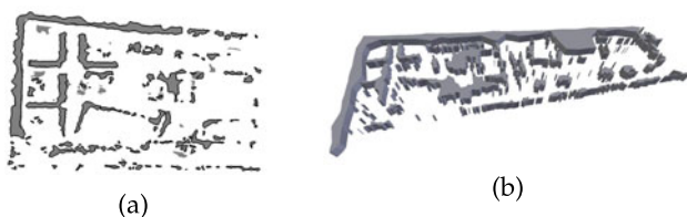
Fig. 8. Navigation meshes generated from 3D models. (a) Navigation mesh of the library area. The gray solid polygons represent the one compiled from the initial 3D model only, while the black hollow polygons correspond to the one utilizing also the user trajectories. (b) The navigation mesh of the CS building updated in March, 2015.
