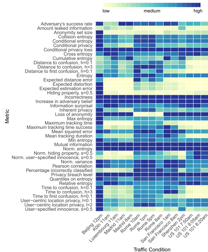
Fig. 12. Heat maps for the shared value range of privacy metrics. The colors indicate the size of the shared value range (from yellow = low to blue = high).
