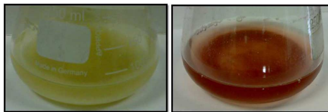
Fig. 1. After 24 h incubation of the actinobacterial isolate in HAuCl 4 medium, the color was changed from yellow to red (left) purple (right).
