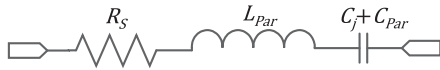
Fig. 2. Equivalent circuit of the varactor diode including the parasitic effects of the package. ( L_{\text{Par}} = 0.4 nH and C_{\text{Par}} = 0.06 pF).
